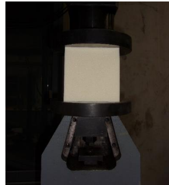
Figura 1: Test setup and load slip example of the Polyurethane characterization – Compression test.
