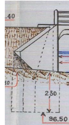
Elevation and view of solid wall abutment with 45° wings floor drawing, 1936 Pocuro Bridge
